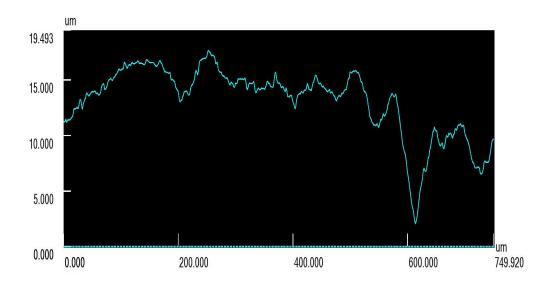
Fig. 9. Distribution of depth values for a crack fragment 750 µm wide according to laser confocal microscopy data.
