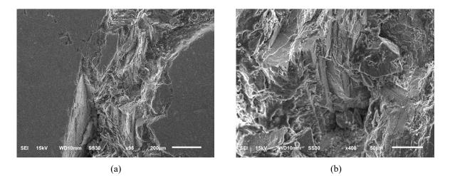
Fig. 8. View of a crack fragment according to electron microscopy. Scale bars: 200 µm (a) and 50 µm (b).
