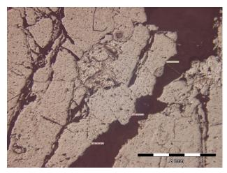
**Fig. 7.** View of a separate fragment of a crack in granite according to optical microscopy data.
